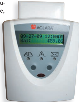
The Pay-As-You-Go in-home display, which plugs into an electrical receptacle in the customer's home, indicates in an easy-to-read format just how much energy is being used.
